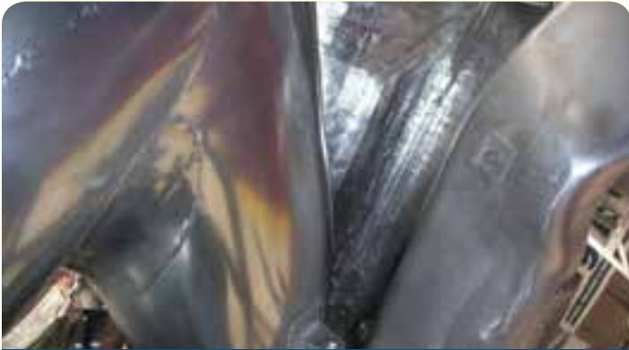
Jay Leno's Eco Jet Car with foil covered ceramic cloth
