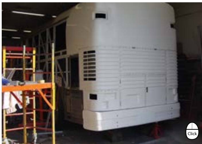
I started skinning the bus in the rear with the rear cap and the entire surround.
