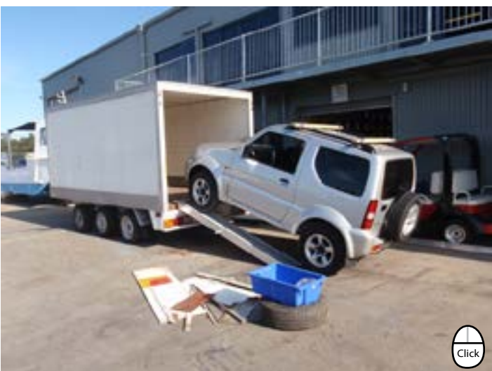
With the three axle trailer, the car can be loaded without trailer being hitched to the bus at the time. Also, GM owners may want to consider this - minimal tongue weight on the hitch.
