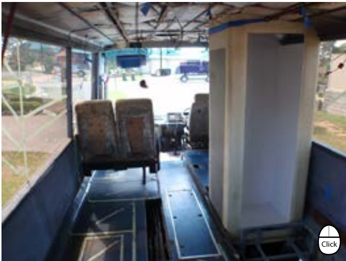
Shower is set into lowered floor section
