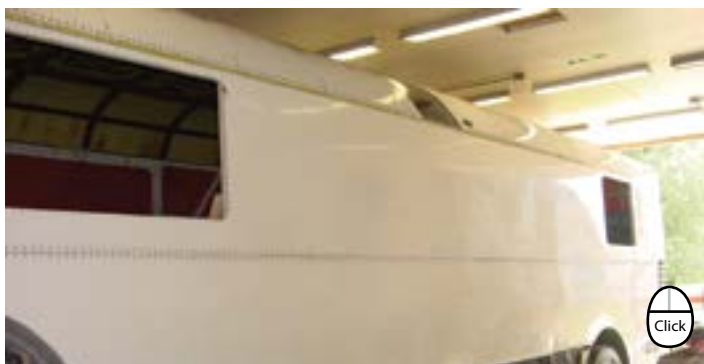
Once the sides were done, I moved to the front cap and then the front surround. The door was skinned next.
