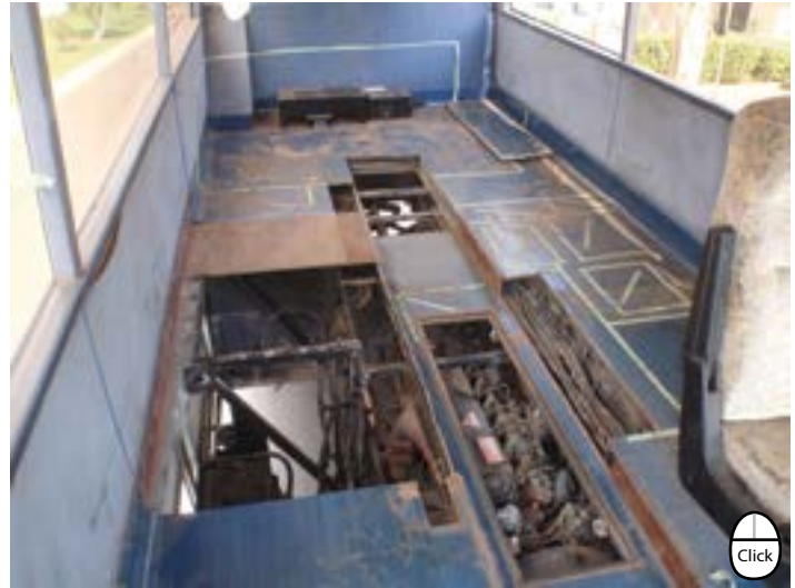
Interior stripped out and floor panels removed in preparation for modifications. Also, you can see in this photo where the engine resides in this mid-engine bus
