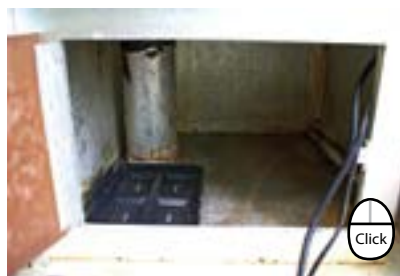
Battery tray in small compartment under the Aqua-Hot. Note the wires on the right. The wires in the split loom are from the switch. The other cable is from the maintenance charger in the electrical bay to the right.
