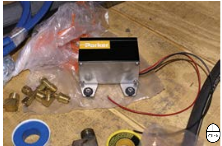
The Parker FPM-50 on the bench with fittings ready to install
