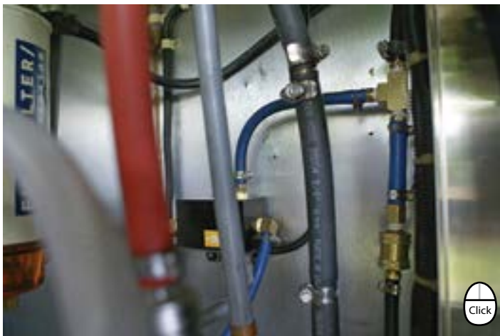
The FPM-50 inserted into the fuel delivery line between the Racor fuel filter / water separator and the Aqua-Hot (horizontal connections). The fuel bypass line comes off the top of the FPM-50 and goes to a Tee in the fuel return line. In polishing mode, the pump draws fuel from the tank through the Racor and returns it to the tank. In normal mode, fuel flows through the FPM-50 as though it was not present.
