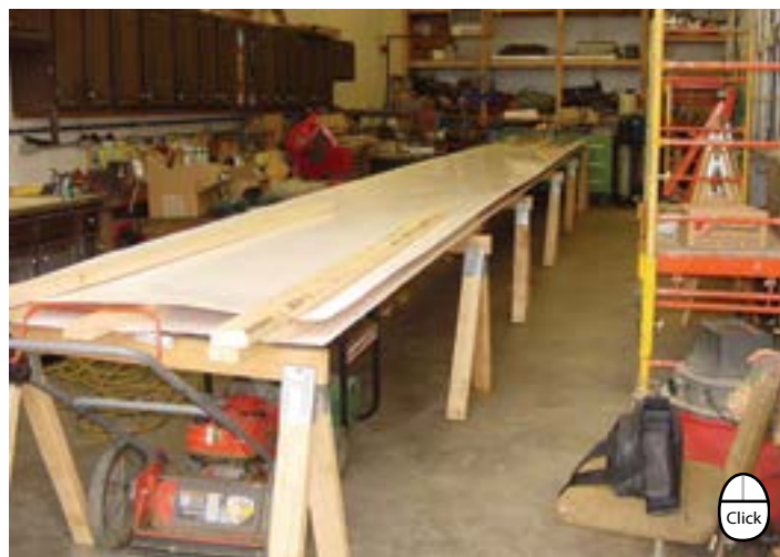
We laid the sides out on sawhorses to flatten them before installation.
