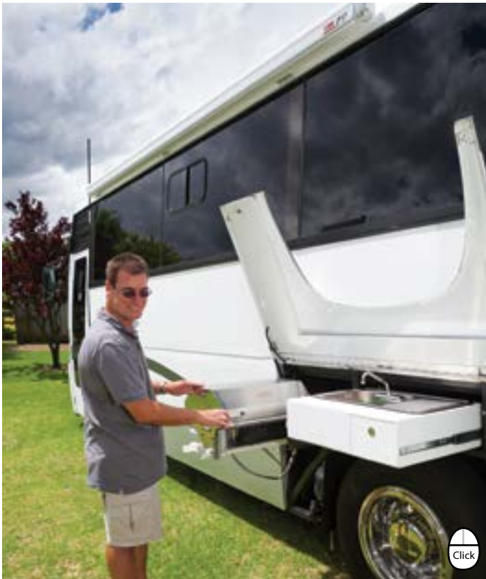
Steve demonstrating the exterior slide-out grill and sink
