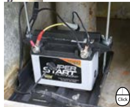
Battery tray in small compartment under the Aqua-Hot. Note the wires on the right. The wires in the split loom are from the switch. The other cable is from the maintenance charger in the electrical bay to the right.
