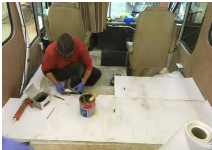
Sylvie piecing together the front steps before covering with 1/2" plywood.
