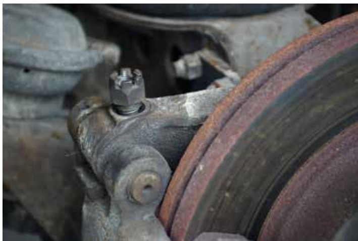
Joe has loosened the castle nut on the retaining pin for the upper caliper slide pin. The retaining pin gets pulled out the top, allowing the slide pin to be tapped out and release one of the two caliper mounts.
