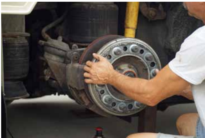
Joe removes the Centramatic dynamic wheel balancer from the driver-side tag-axle hub.
