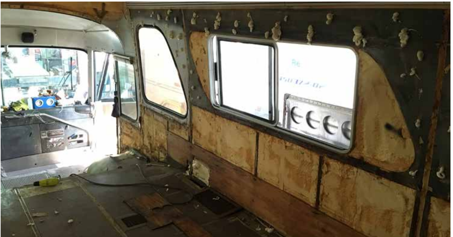
Spray urethane insulation that was already in the bus.
