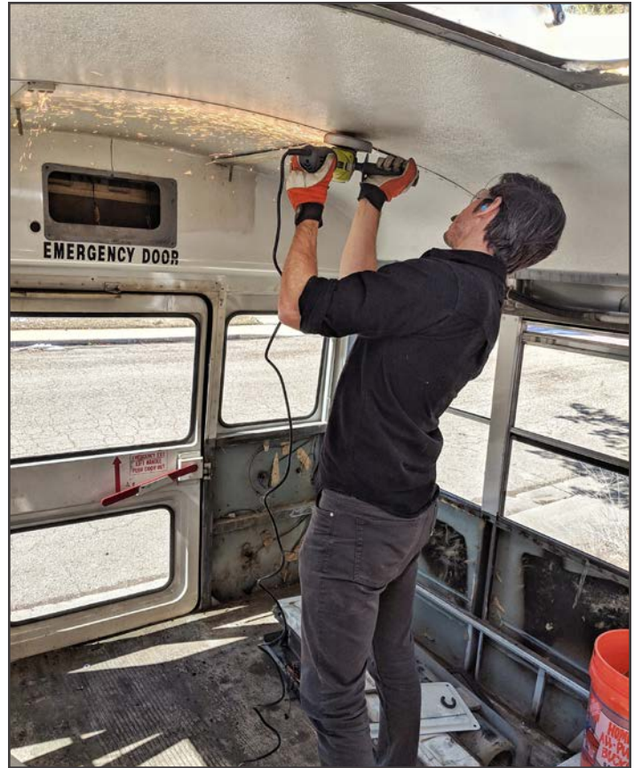
Demo time! Cutting the thousands of rivets off to get the metal roofing down.
