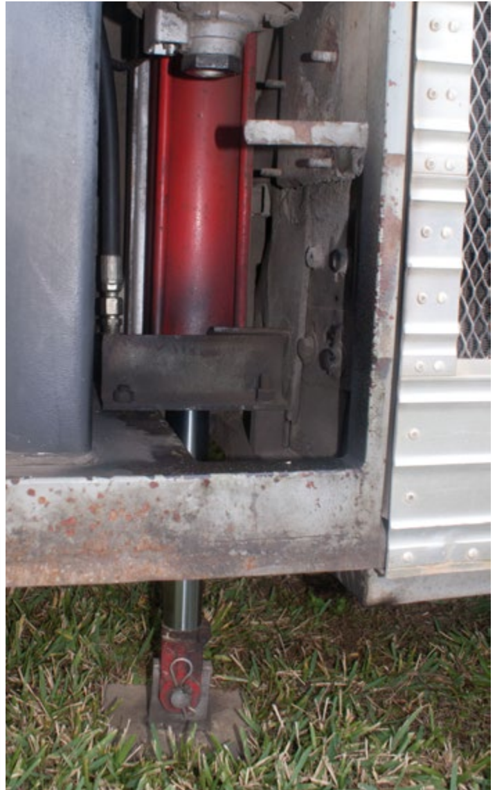
One of the four hydraulic cylinders used to level Iron Horse
