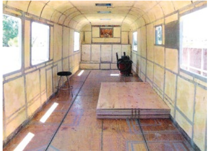
With the insulation completed, the interior is ready for the building work to start. Notice the outlines on the floor. This is an important part of the planning phase. It is a lot easier to move something when it is just a mark on the floor.
