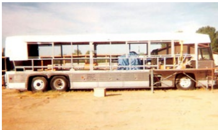
We raised the roof and installed new front and back caps to make room for insulation, air ducts, .
