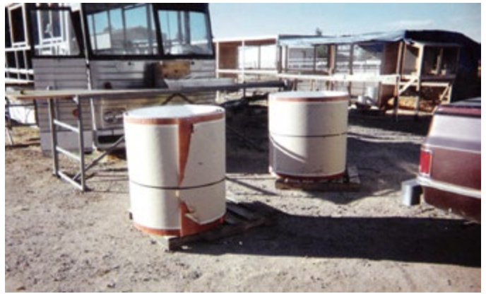
Rolls of fiberglass panel ordered for reskinning the sides of our bus after the roof raise. This also facilitates installing RV style slider windows.
