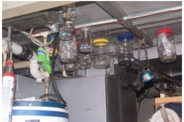
Small hardware is organized and stored using jars attached to the ceiling of the cargo bay.
