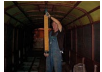
Guide with one hand on drill, feed the drill by pulling up from bottom
